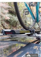
This fork-mounted rack carries a load of up to 40 pounds, and it's adaptable to both mountain bike and narrow road bike tires. The rack's skewer fits both quick-release or thru axles, adding to its versatility. And the rack's lever-strap system adjusts quickly, adapting to aerodynamic, round, or square crossbars.
