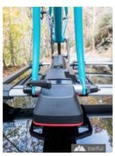
The Yakima HighSpeed solidly solves those problems thanks to its innovative design. Mounting the bike is simplified: nearly half of the mounting work can be finished at ground level, since the rack's axle and skewer can be mounted to the fork while it's still on the ground. And then mounting the bike to the rack is simple: a few turns of the large, easy-grip torque knob secures the fork to the front of the rack, and a strap secures the rear wheel into the wheel tray.
