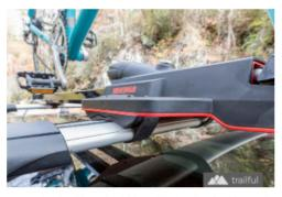
Mounting the HighSpeed to crossbars is tool-free and straightforward, thanks to the adjustable straps that wrap securely around the vehicle's crossbars, and then lock into place with a combination lever and slide. Fitment adjustments to the vehicle's crossbars are made with the turn of a tension thumbwheel – and make moving the bike rack between multiple vehicles and multiple crossbar types easy.
