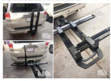
Admittedly, the most frustrating part about the installation process was snapping the snap ring into place. I just couldn't do it. Holes at the end for a snap ring were absent, and I don't own a snap ring tool. So, armed with my friend's needle nosed pliers, I was eventually able to seat it.
