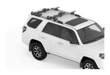
The Yakima ShowDown is a lift assisted product designed to help owners get their kayaks or SUP onto the roof of the vehicle. The Showdown lowers the mounting level two feet and supports up to 80lbs.
